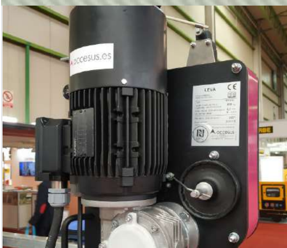
NFC tag on the Accesus LEVA electric lift.
