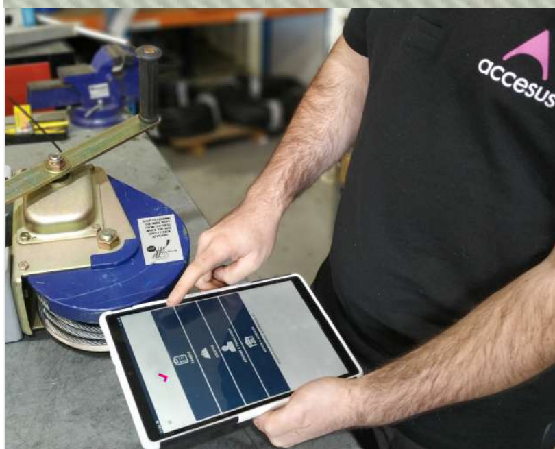
Accesus personnel carrying out an inspection of a lift-rescuer with V.acces software.
