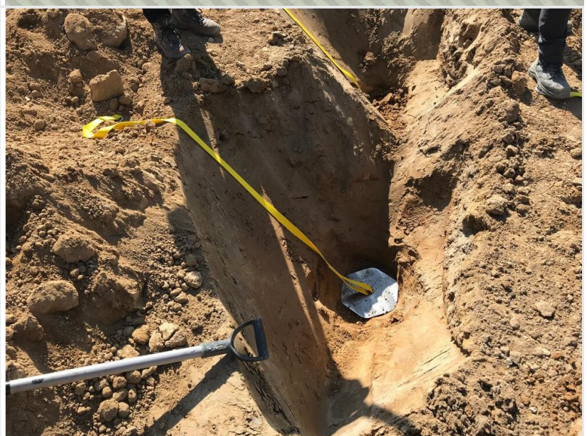
Practical application of the PAT 189 anchor point in the field.
